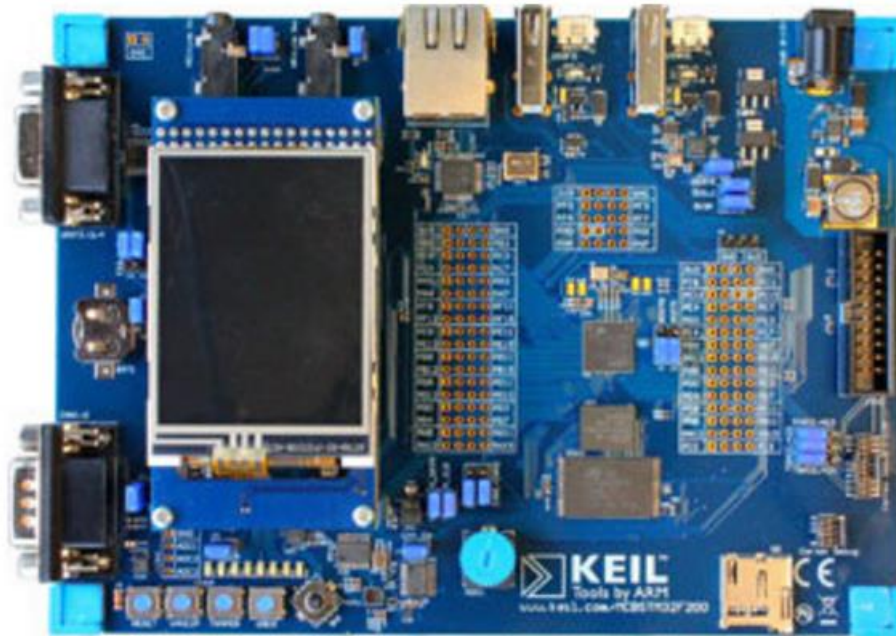
Figure 1. Oracle's Java ME Embedded 3.3 will run on platforms like Keil's STM32 F200 Evaluation Board with 120 MHz Cortex-M3, 1 Mbyte of flash memory and 128 Kbytes of RAM.
